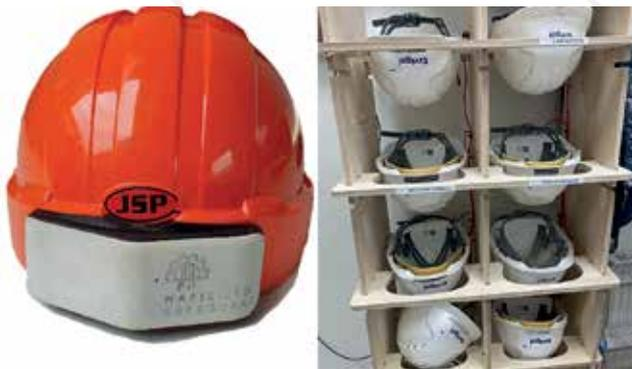
Figure 2: Mafic device and charging station
