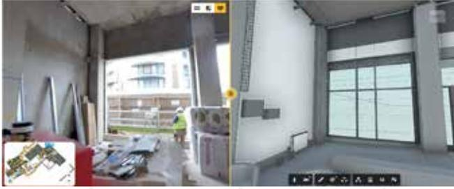
**Figure 9:** One click connection to BIM model for any scene in the Virtual job walk, with synchronised navigation within the 360° frame.
