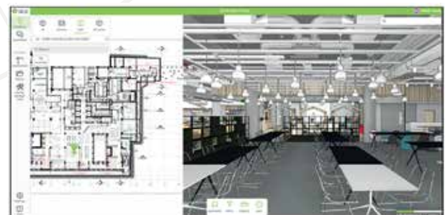
Picture 1: Dalux BIM Viewer layout, familiar 2D drawings brought to life within the 3D environment.
