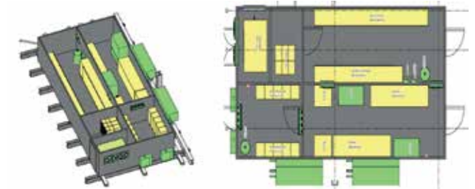
Figure 5. Containerised Electrical Plant Room Typical Example
