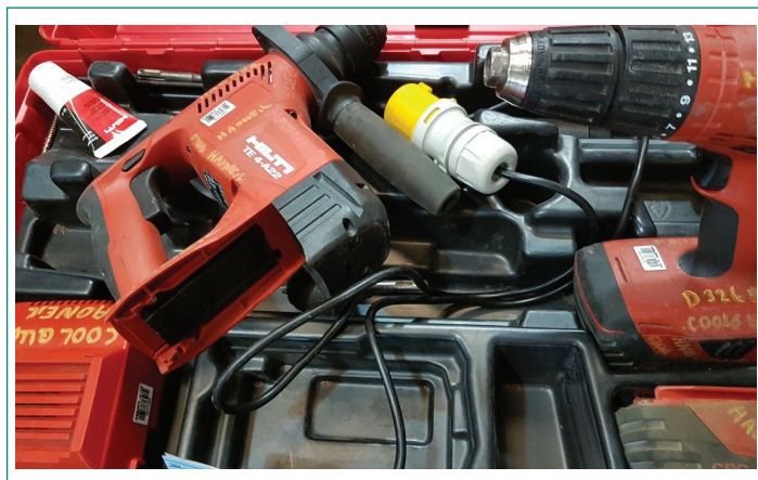
Figure 2. Tools Displaying Barcode Tags
