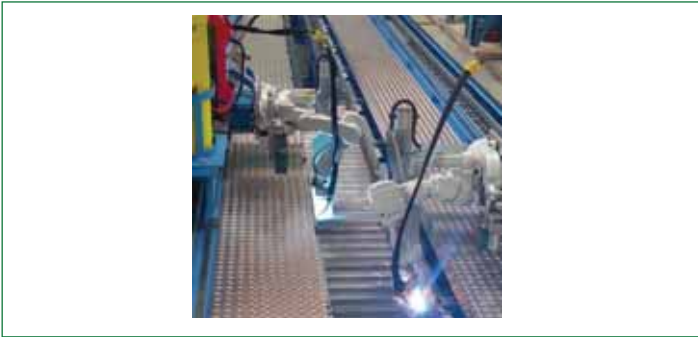
Figure 2. SIN Beam Robotic Welding.
