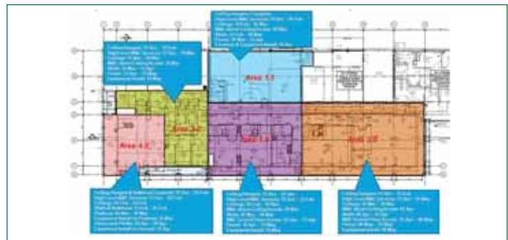
Figure 5. Graphical Representation of Cleanroom Coordination with MEP Trades.
